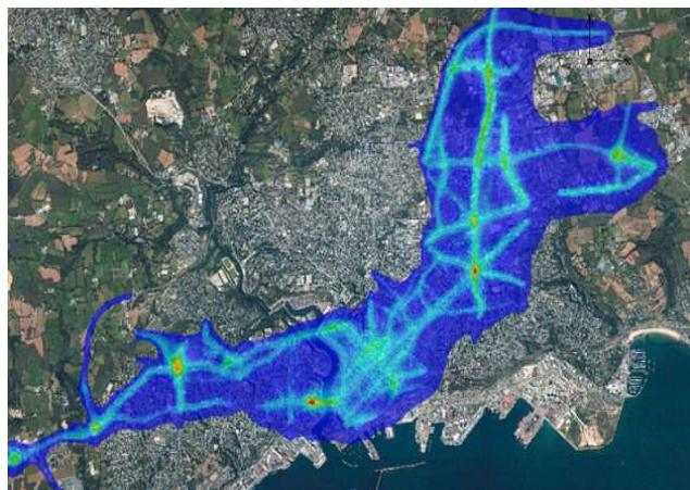
The results of the calculations are displayed on a background map in the form of colour concentration contours, concentration profiles on traffic routes, wind fields etc.
