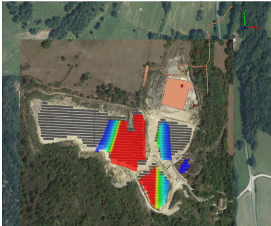
3D Modelling of Dust Dispersion from a quarry
