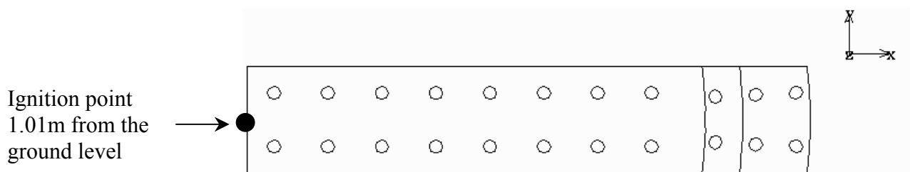
Fig 4: The ignition point.
